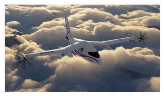
The five-passenger Alycon M3c is planned to be hybrid-electric initially, then hydrogenpowered.
