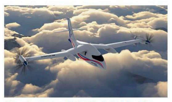
The six-seat Alcyon will use the same hybrid propulsion components as the tandem-seat Alerion, in a distributed, redundant configuration.
