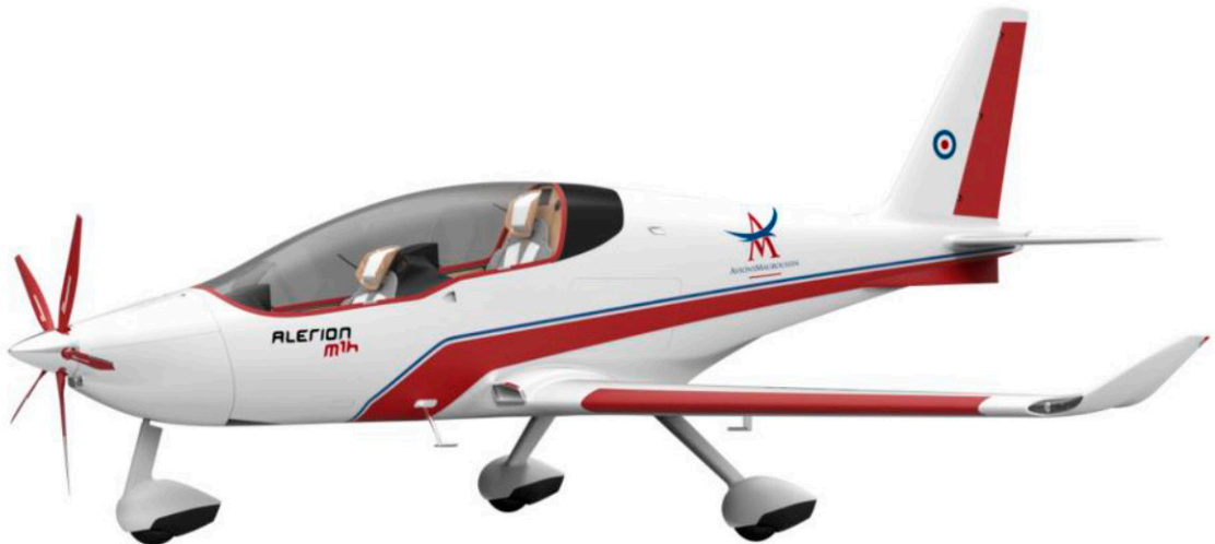
The two-seat Alérion M1h is one of two hybrid eSTOL aircraft being developed by France's Avions Mauboussin. (Image: Avions Mauboussin)
